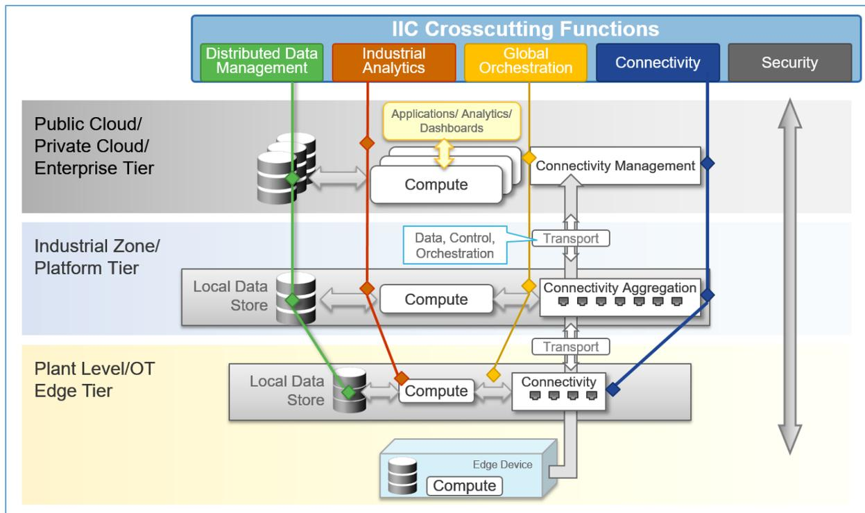
Figure 1: IIC Crosscutting Functions Across Edge Computing Architectures
