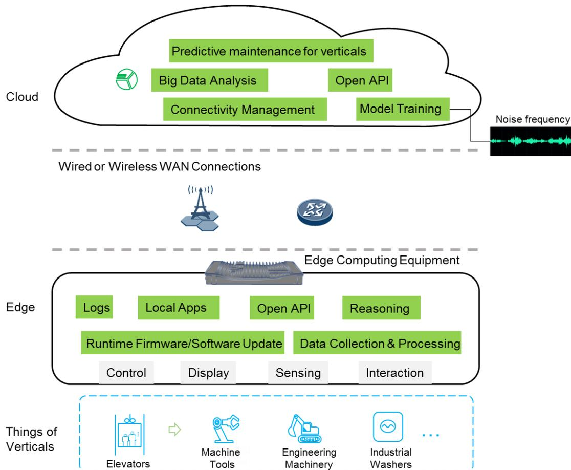
Figure 6 Logical Architecture Diagram for Edge Computing
