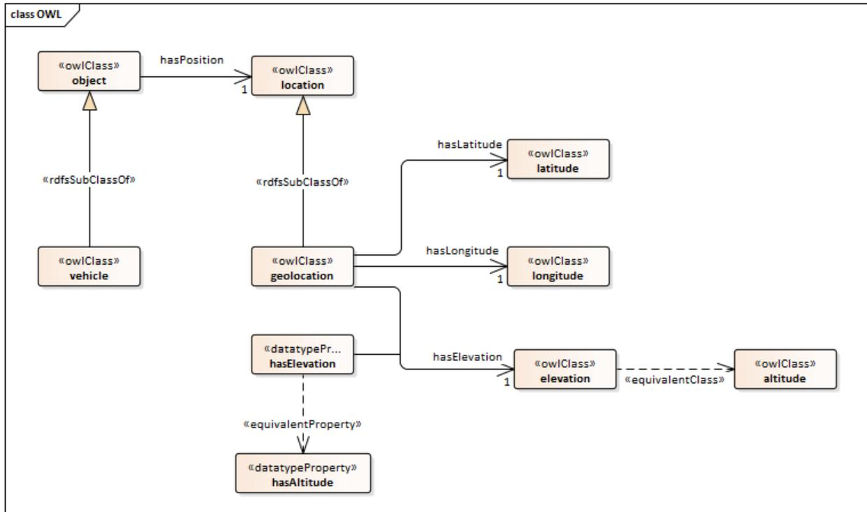
Figure 6: ODM Representation of Vehicle Location
