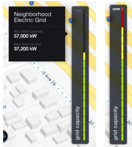
Figure 6: Electric Grid capacity before and after adding panels and arrays
