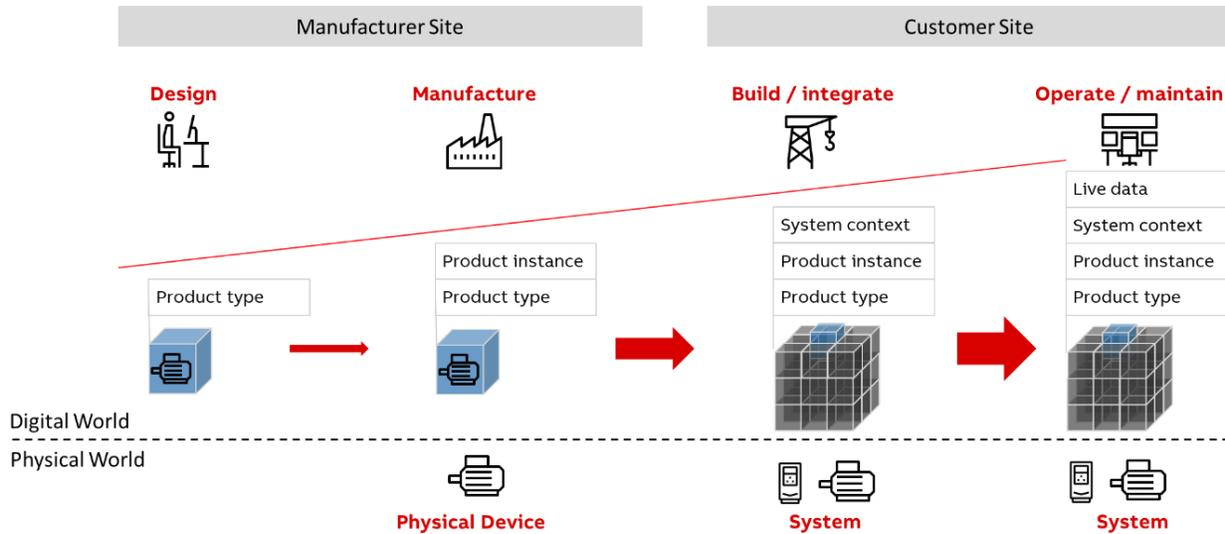
Figure 5: How Digital Twins can tackle the Information Silo Problem (ABB)
