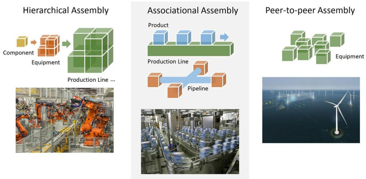
Figure 4: Relationships between Digital Twins in an Assembly (Yo-i Information Technology)<sup>4 5 6</sup>
