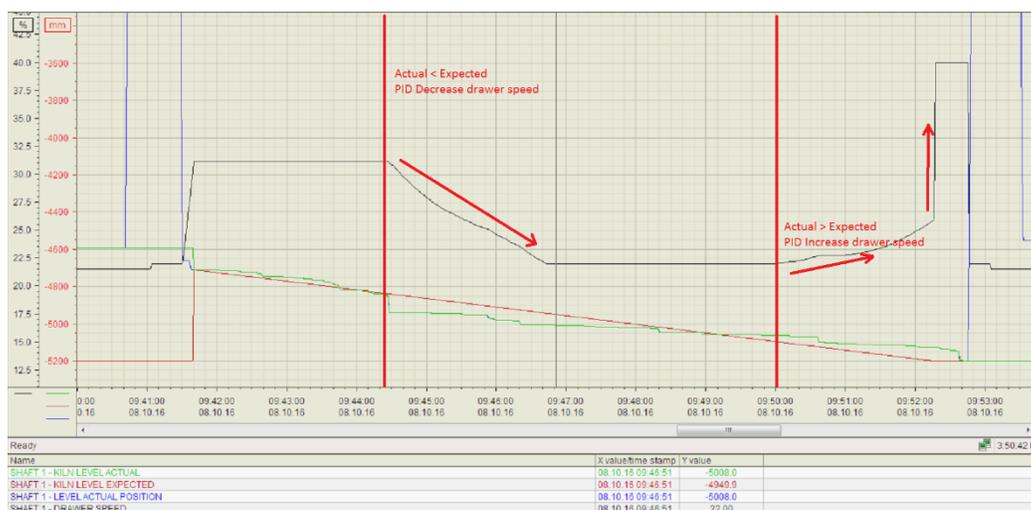
Figure 4 Typical discharge system PID cycle
