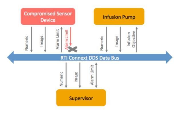
Figure 7. Simplified Architectural Diagram of OpenICE Infusion Safety App
