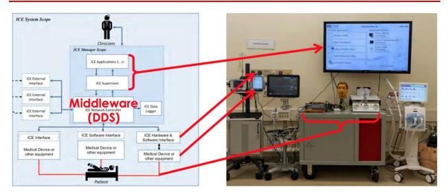
Figure 1. General architecture of ICE and an instantiation of it in a test setup at MD PnP Lab.
