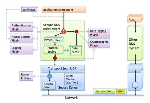
Figure 2: Architectural View of DDS Security
