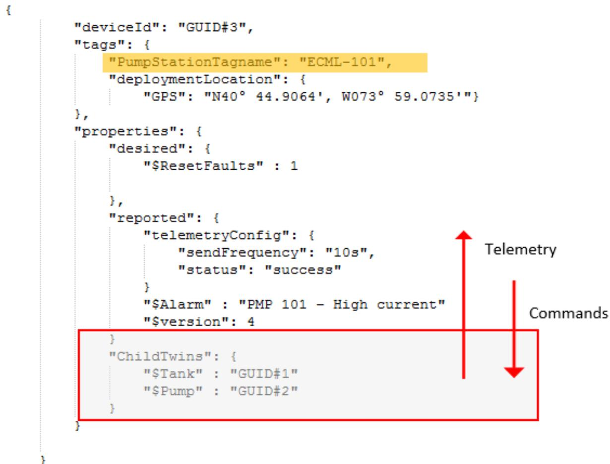
Figure 5 Pump Station JSON Digital Twin model
