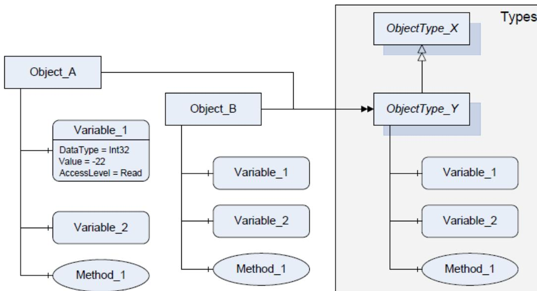
Figure 7 OPC UA representation of an object
