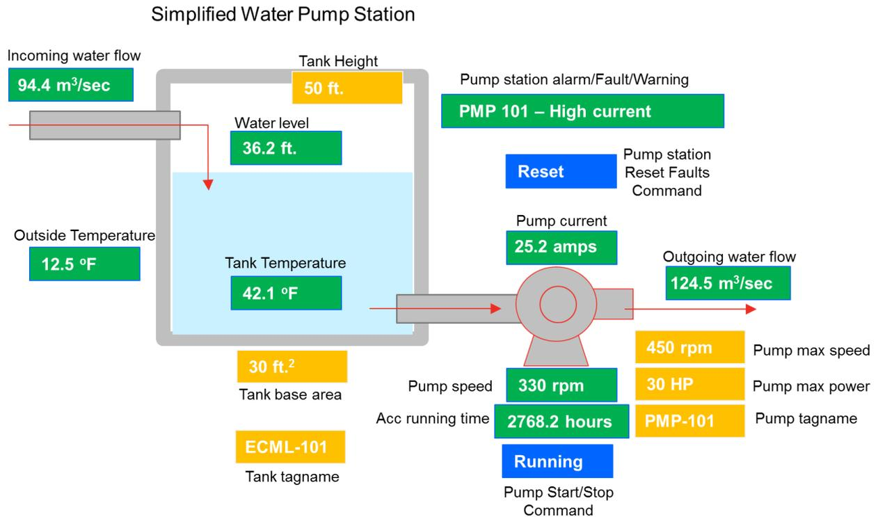
Figure 2 Modeling digital twin for a water pump station
