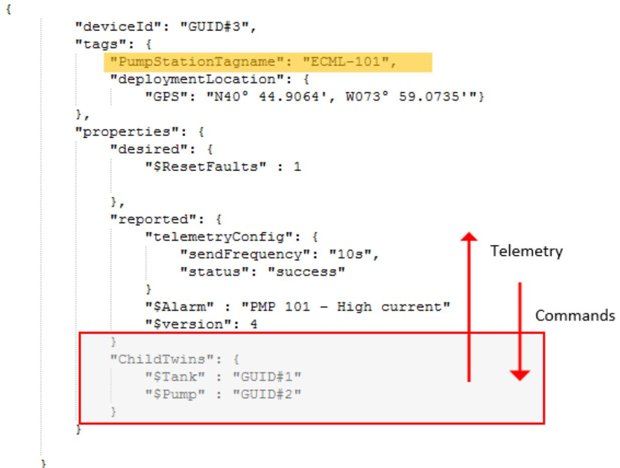
Figure 5 Pump Station JSON Digital Twin model
